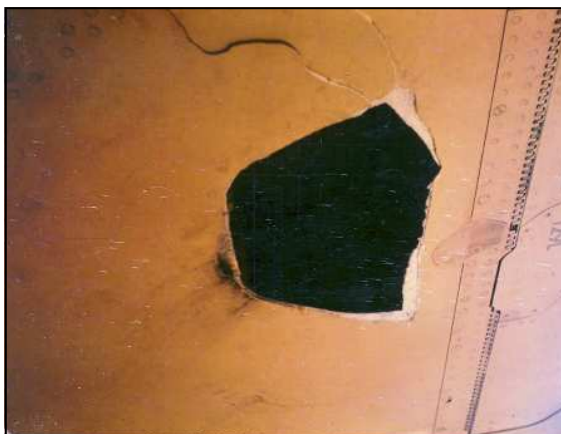
The hole in the wing of Major Richard Starke's RF-4C.
